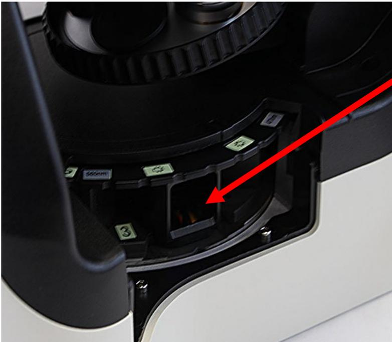
2. Shown here, the filter cube is properly seated and installed.
