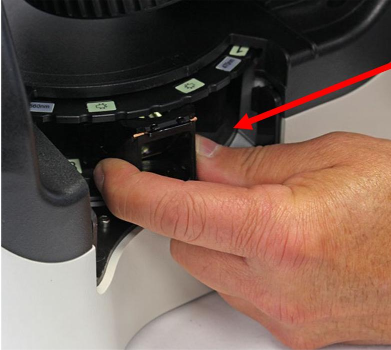
1. To install a filter cube, align the cube notch with the securing pin on the inside right of the turret receptacle and carefully slide the cube in until it clicks into place.
