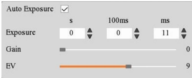
**AUTO EXPOSURE:** Check [Auto Exposure] to automatically adjust the exposure time.
