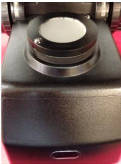
This component is comprised of two flanges; a semi-permanent mounting flange and a swing-in diffuser. The lower flange has a four-tooth bayonet arrangement. Placing it on the light port as shown below will allow it to seat down onto the light port.
