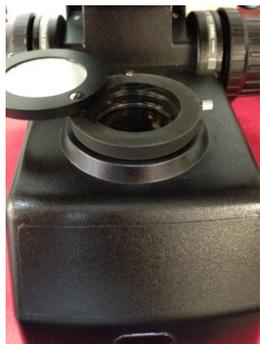
To temporarily remove the diffuser from the light path swing the upper flange CCW.
