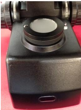
Next the assembly is rotated 45 degrees. This will engage the bayonet teeth. When correctly installed, the thumb screw on the lower flange should face 3 o'clock. Lightly tighten the thumb screw.
