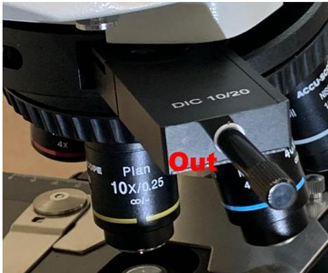
5. With the analyzer facing up and the metal knob oriented out, slide the analyzer into the slot. The analyzer attaches to the slider with magnets and uses a pin that fits in a slot on the slider to ensure correct orientation (and not a 180° rotation)
