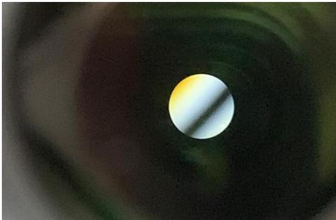
7. While looking down the eyetube without the eyepiece, turn the Analyzer/Slider control knob until a dark line is observed in the rear of the objective. The line will be at a slight angle, running from southwest-to-northeast.
