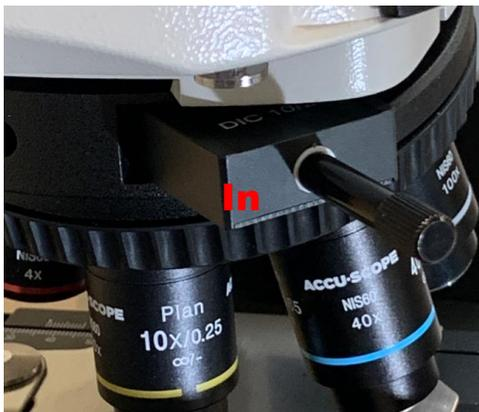
*Note that there are two stop positions on the slider. For DIC observation, push the slider all the way into the slot. For brightfield observation, gently pull the slider out until the detent clicks into place, and this is the “out” position. The slider does not need to be completely removed from the nosepiece for non-DIC observation (e.g., brightfield or fluorescence) and can remain in the out position.*
