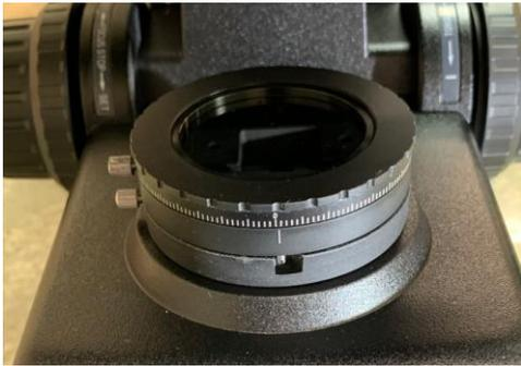
3. Set the rotatable polarizer ring to "0" degrees.
