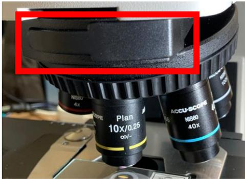
4. Remove the dust plug (red box) from of the nosepiece to open the analyzer slot.
