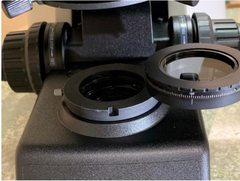
1. Place the polarizer attachment on the light port of the microscope base with the locking thumbscrew oriented to the left side at 9 o'clock position.
