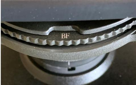
6. Rotate the condenser turret to the BF position.
