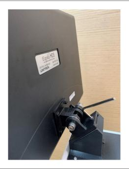
Attach the monitor to the mounting block using the two (2) black 16mm screws and 2.5mm hex tool provided.
