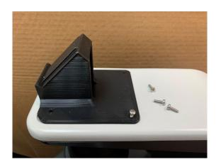
Install monitor mounting block using the longer screws provided with the mounting block.
