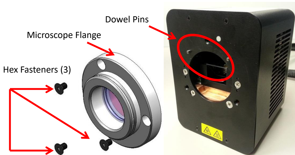
Figure 4 Installing Microscope Flange on LED Head
