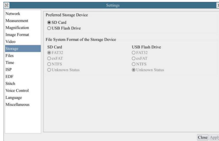
Figure 16 Comprehensive Setting of Storage Page
